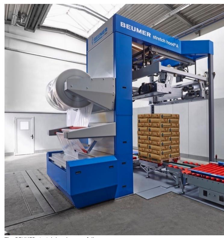
The BEUMER stretch hood covers full pallets with a thin film hood. This ensures that the packaged products reach their destination undamaged and are well protected against moisture and weather influences.
