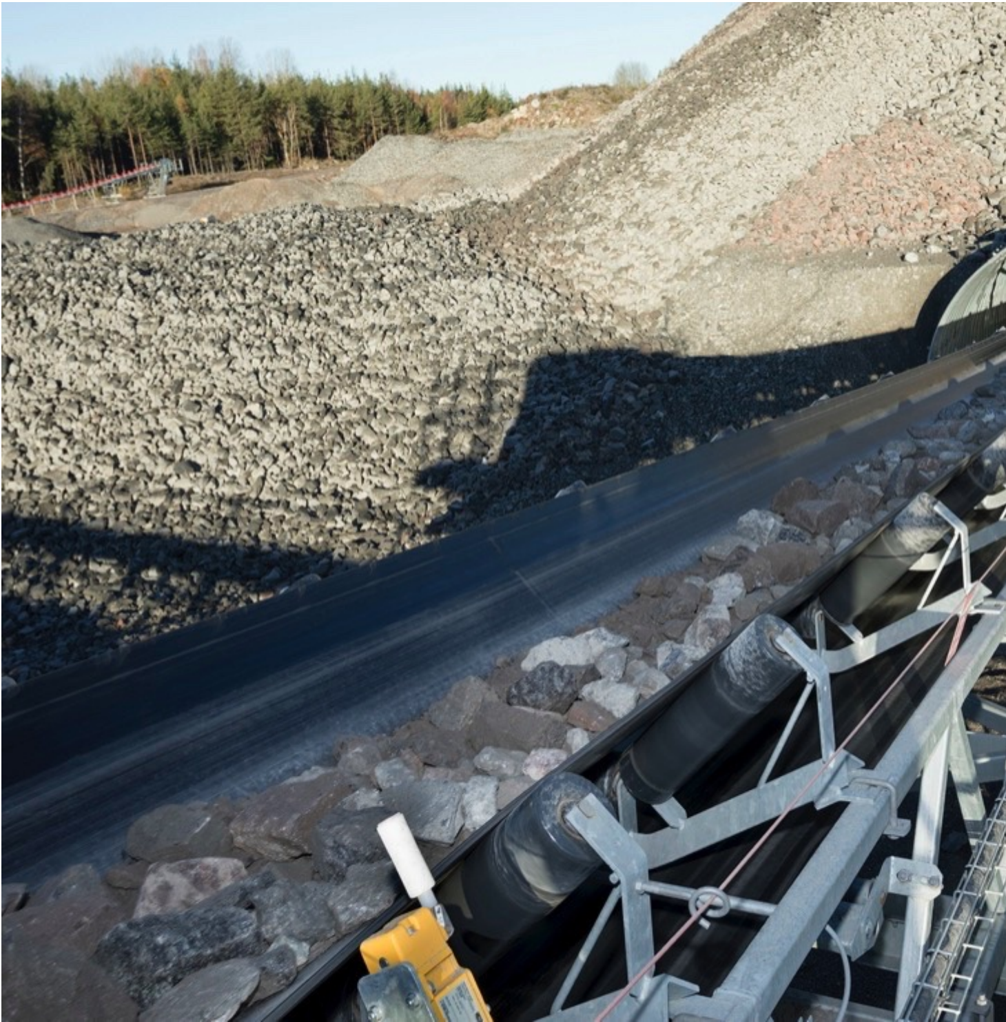
At Jehander's quarry, Continental conveyor belts are being used for the smooth transportation of rubble from the Stockholm mega-tunnel so that it can be reused for the road construction requirements involved in the infrastructure project. (Photo: Continental/Börje Svensson)
