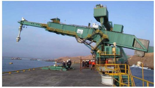
This photograph shows a TAKRAF ship loader for for copper and zinc
