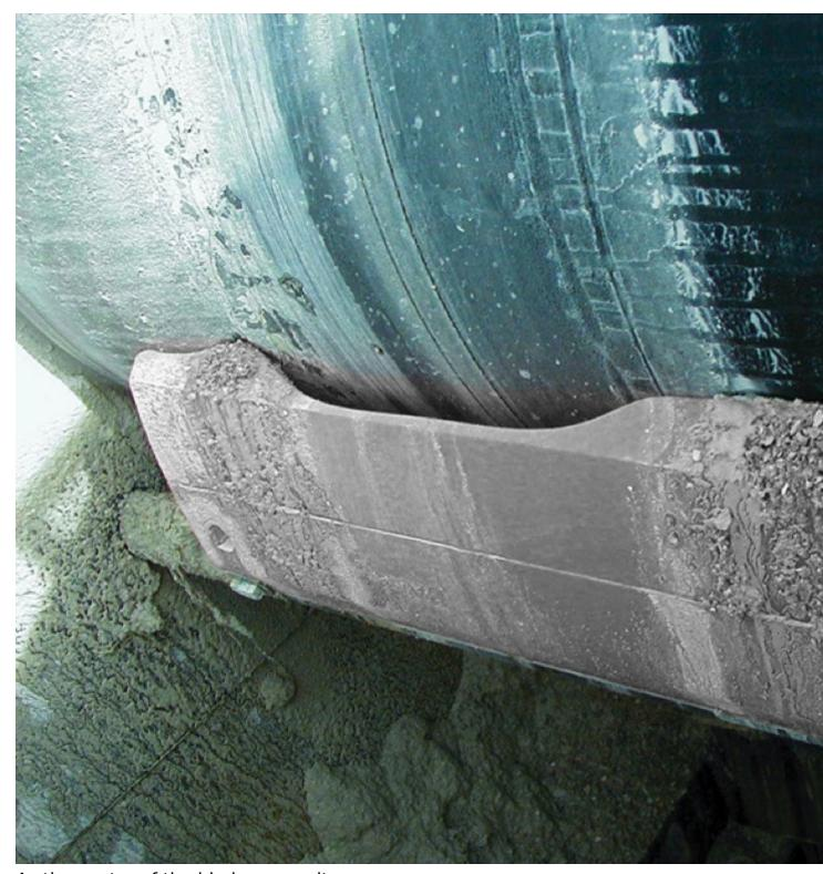
As the center of the blade wears, it allows material to pass inside the tip; the outer edges will be held away from the material and so do not wear.
