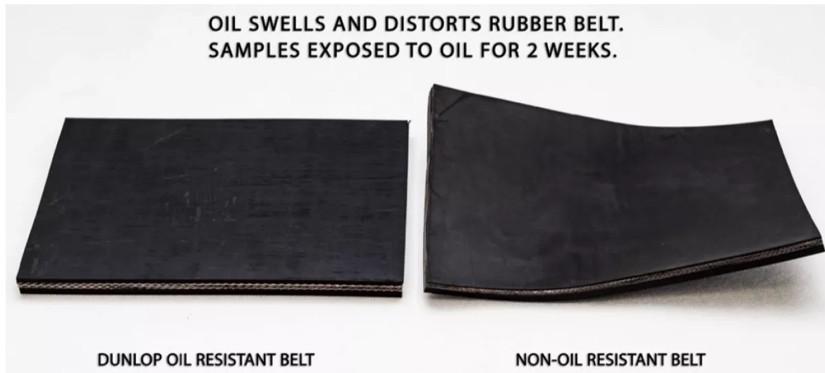
Belt samples following oil test.
