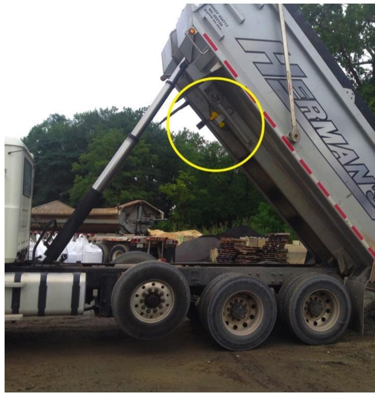
The Cougar DC 2500 vibrates the frame spine, which agitates the material adhered to the bed.
