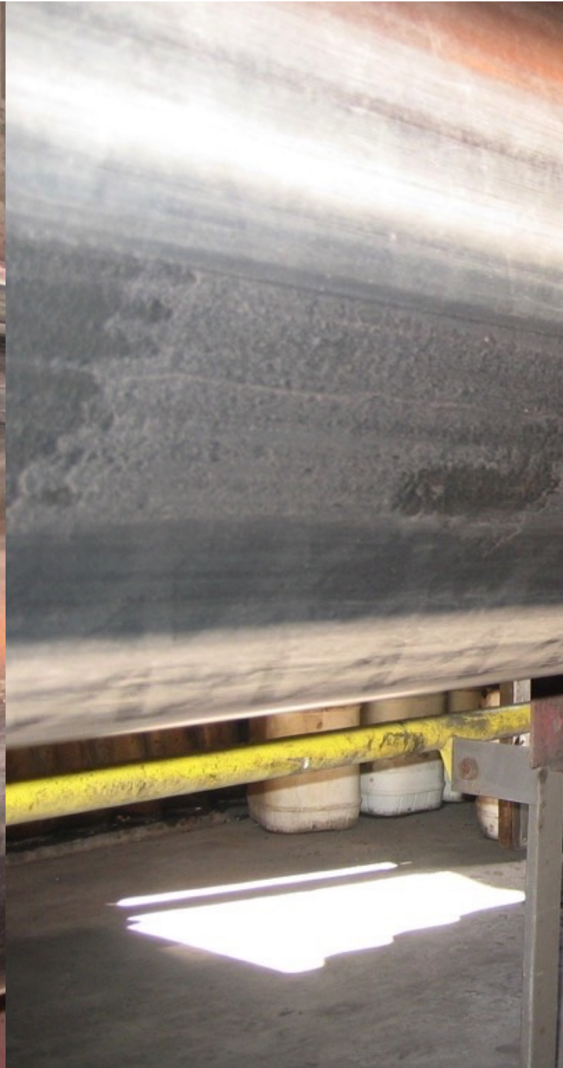
Fig. 13: Also in the return strand the belt contacts all idlers.
