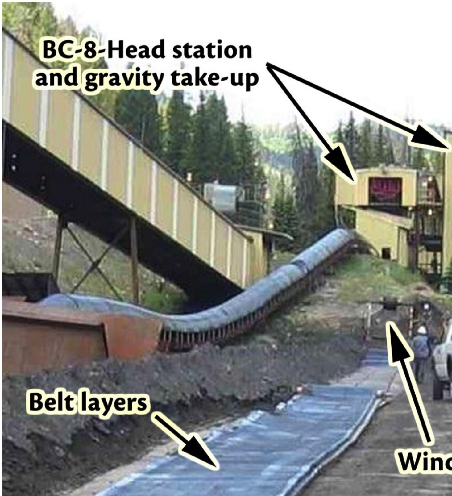
Fig. 7: Reeving of the belt with a winch.
