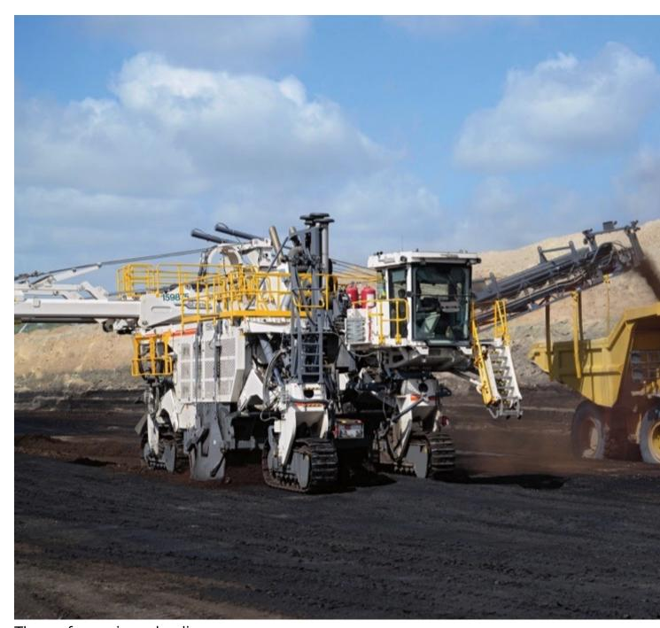
The surface miners loading conveyor can be slewed 90° to either side.
