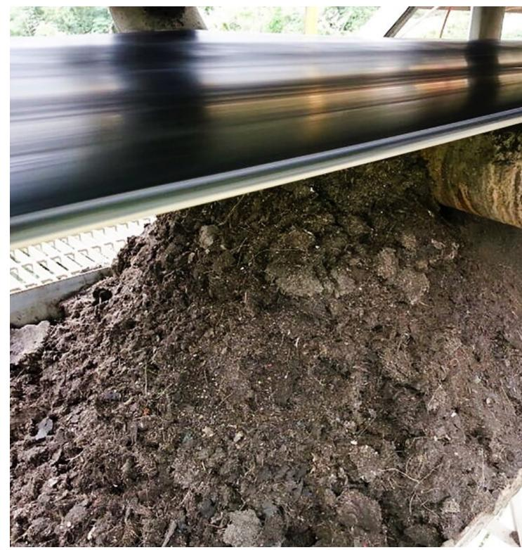
Fugitive material caused equipment failures and maintenance costs estimated at USD 67 000 per month. (Pictures: © Martin Engineering)
