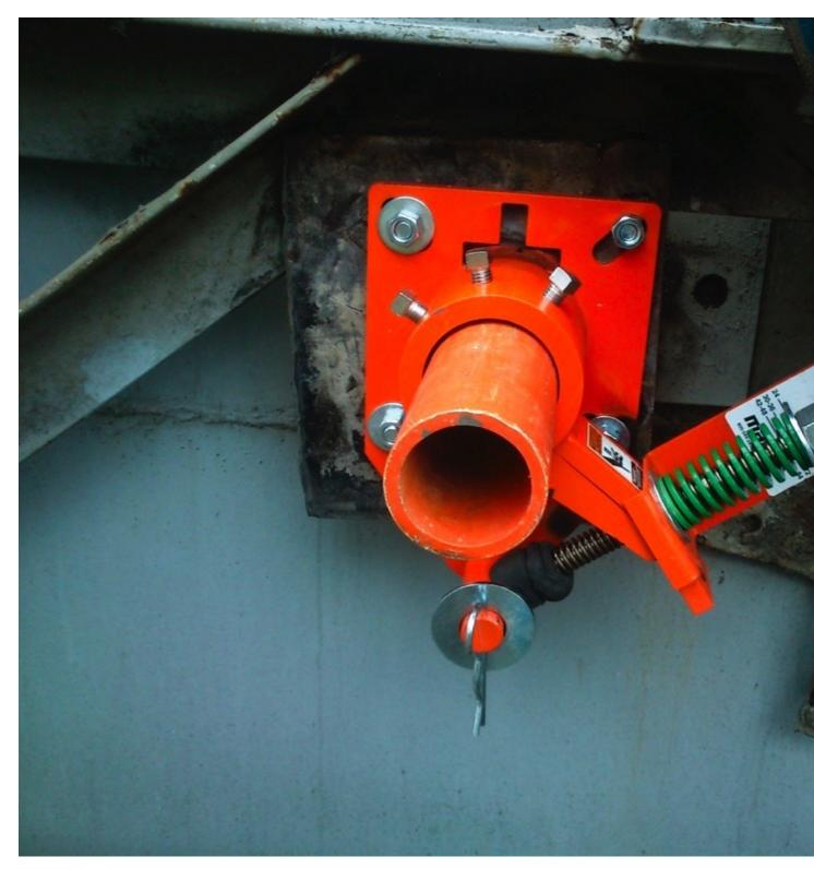
The single urethane blade is mounted on a steel mandrel and tensioned with a heavy-duty spring.
