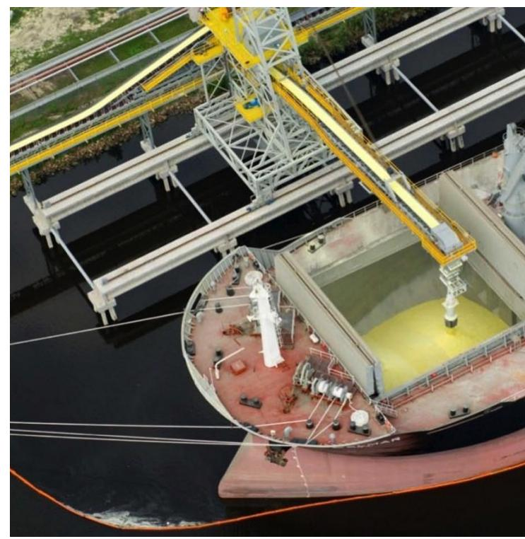
The new Siwertell ship loader will be used for loading prilled sulfur at a rated capacity of up to 1200 tph. (Picture: © Bruks Siwertell)
