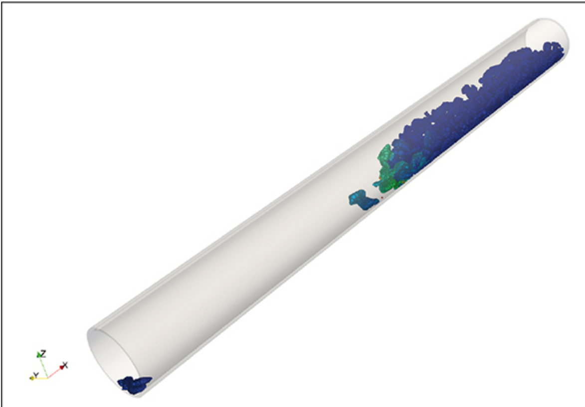
Fig. 12: Material starts sliding back during the emptying of a Megapipe with and without 50-mm-high chevron cleat ribbing in the DEM-FEM model: max. angle of incline is 29^\circ and 46^\circ with the smooth Megapipe and the Chevron-Megapipe respectively. (Picture: © Contitech AG CBG)
