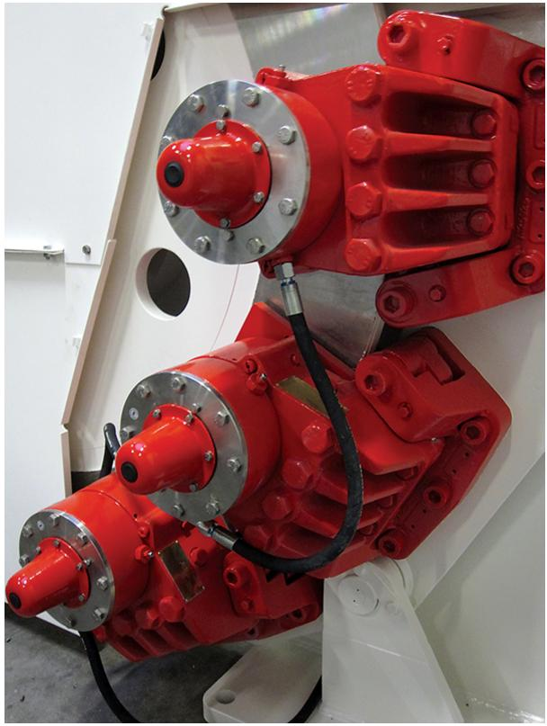
If the brake is to be used for static holding then bedding in may not be possible so engineers should allow for reduced friction potential in the original design
