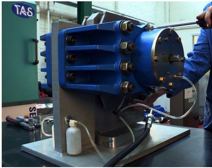
Twiflex offer a 'Parked Off' feature which removes potential energy from the brake during maintenance and allows for brake force to be easily adjusted.
