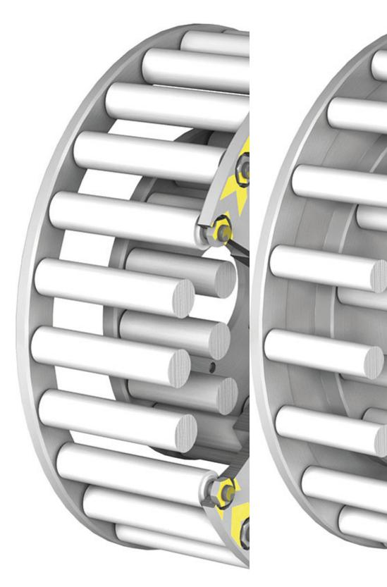
The cages are arranged concentrically, with each row spinning in the opposite direction from that of the row adjacent to it. The material to be reduced is fed into the center of the innermost cage, where it is struck by the massive spinning pins .
