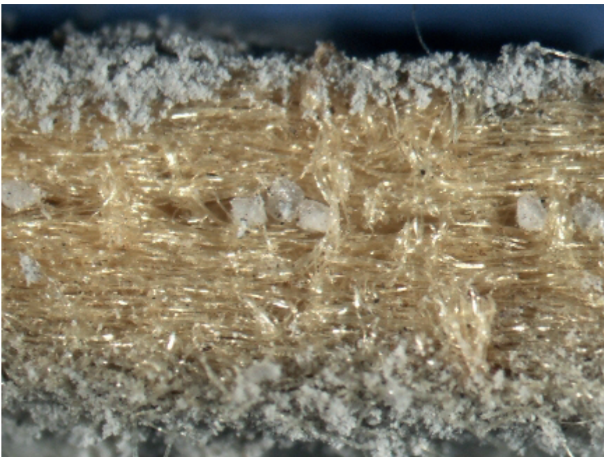
Fig. 4: Contamination from the clean gas side.
