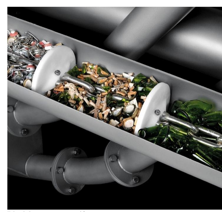
Tube chain conveyors are used for powders or sludges as well as for hard and even abrasive materials such as glass bottle scrap. (Pictures: ©Schrage Conveying Systems)
