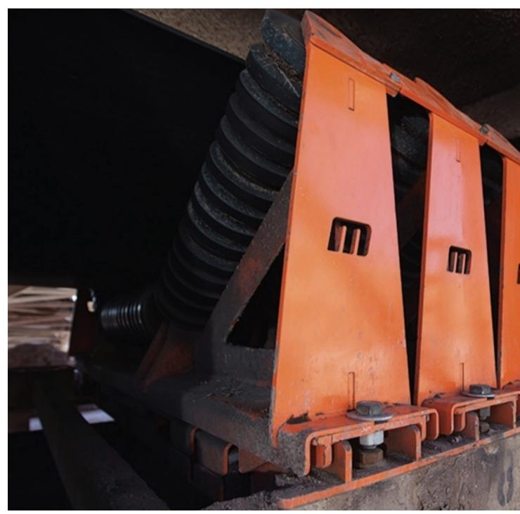
Track-mounted idlers allow easy access for quickly swapping out seized rollers.
