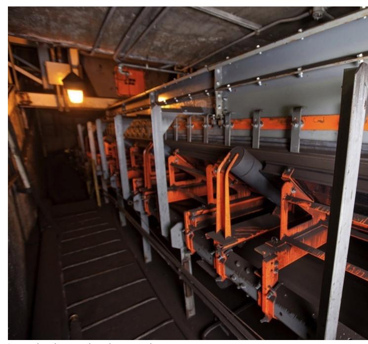
Inspection doors and track-mounted components facilitate maintenance for extended equipment life.
