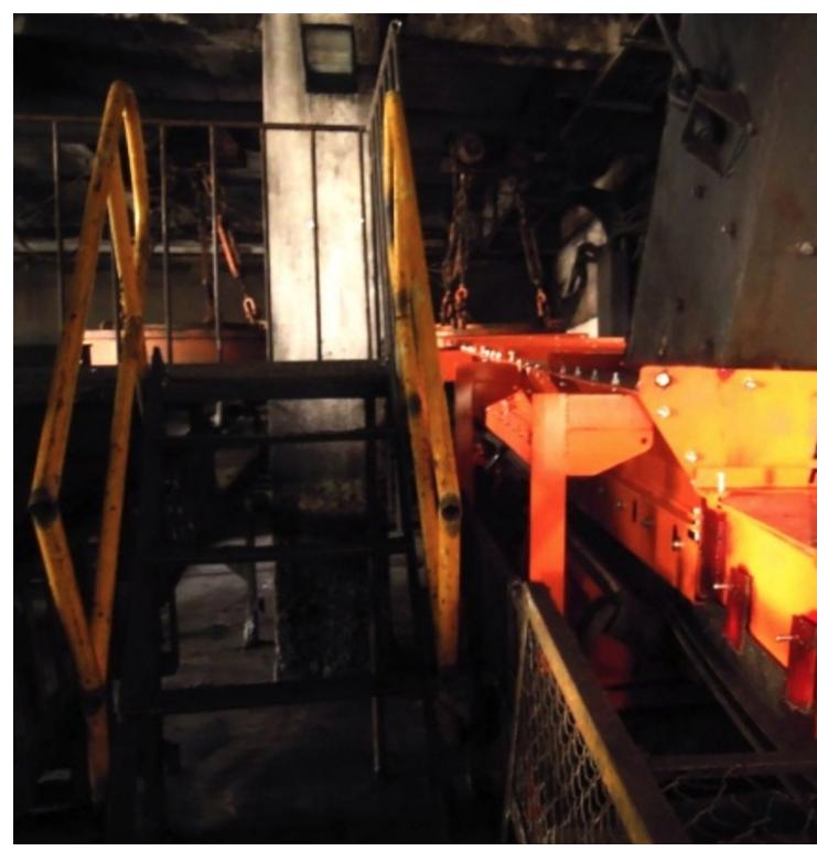
A hatch over the tail pulley allows staff to easily detect entrapped material.
