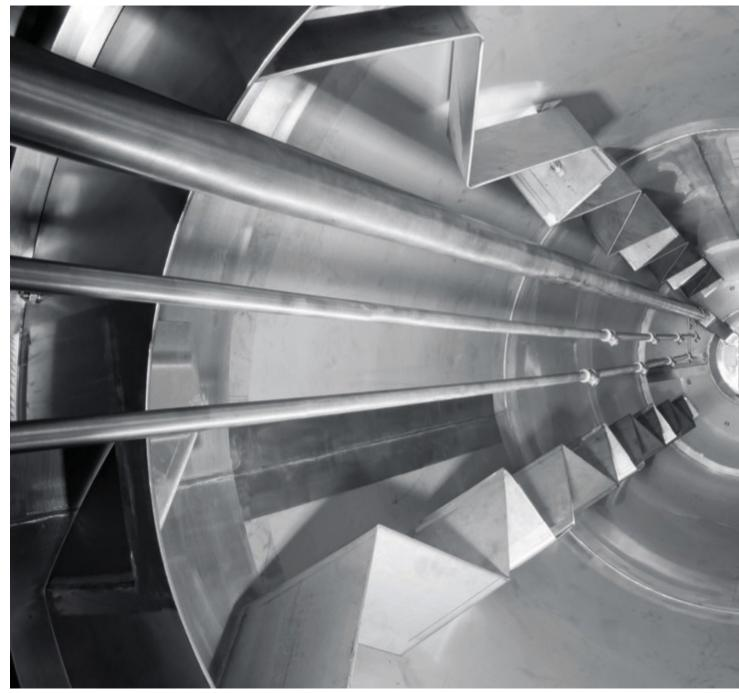
As the drum rotates, proprietary mixing flights distribute particles rapidly with no shear. Optional internal piping (left) feeds nozzles that coat cascading material with liquids.
