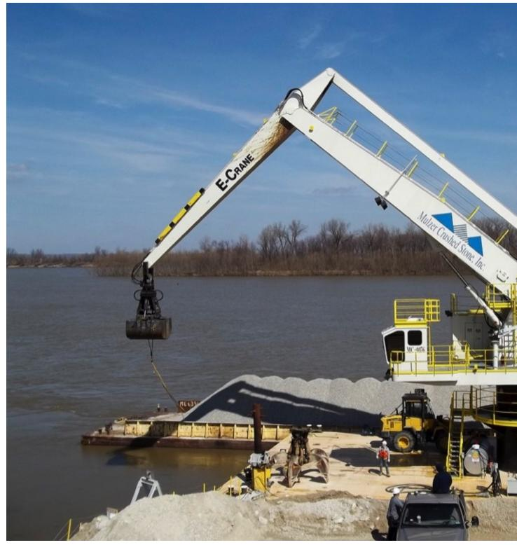
The E-Crane balanced design makes it ideal for barge mounting. (Pictures: © E-Crane)
