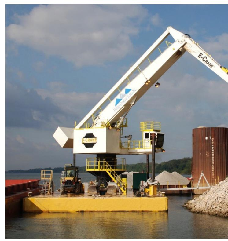
A 1500B / Model 11264 E crane with a grab capacity of 16.5 t and an outreach of 26.4 m. The Mulzer-crane will be barge mounted.
