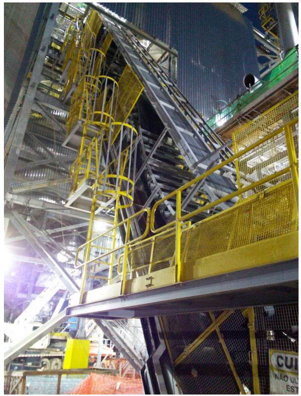
The DSI Sandwich belt high angle conveyor offers a small footprint elevating 720 t/h of limestone, iron ore, sand and clay at a 60 degree angle.
