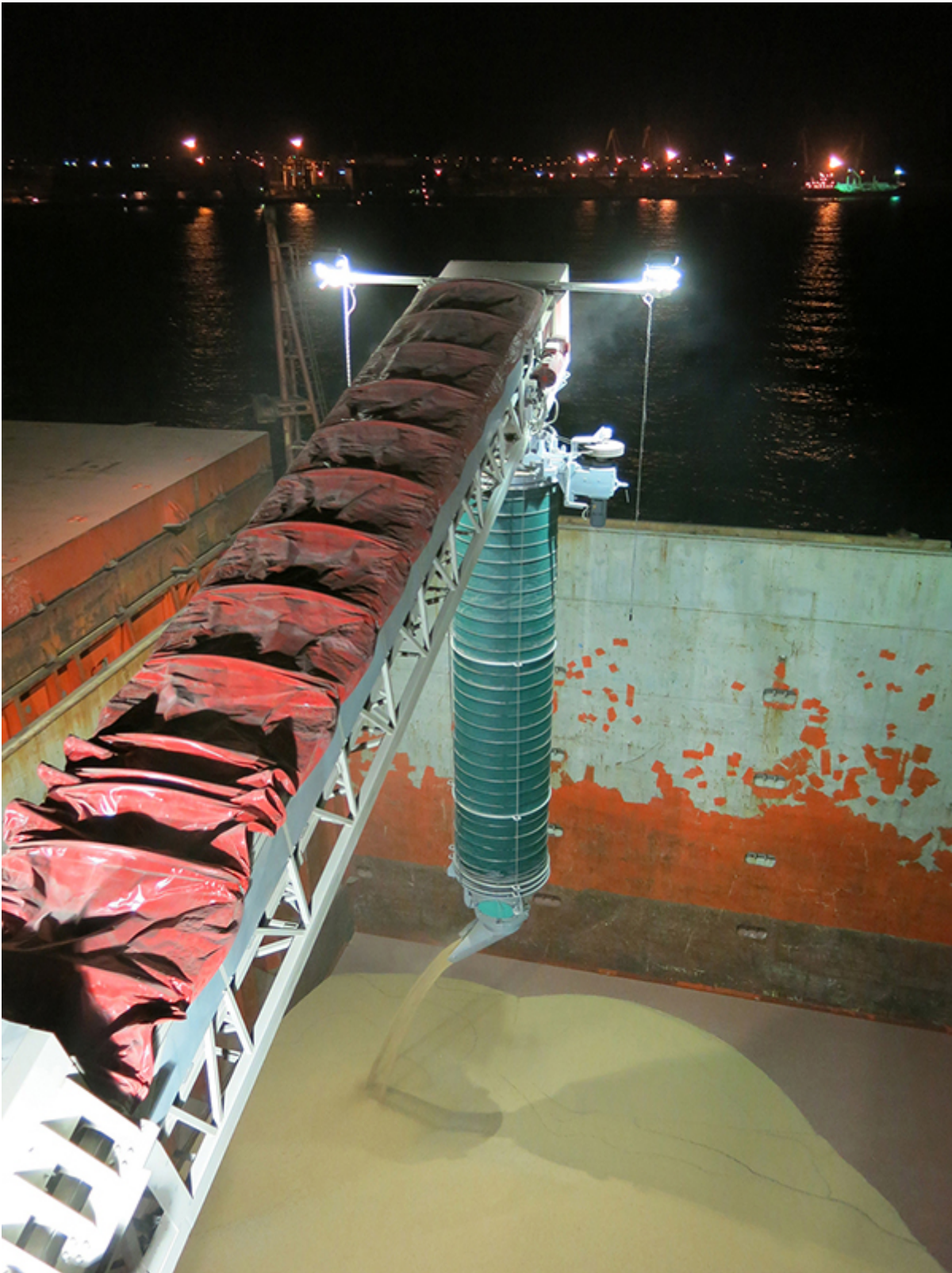
TelestackTS 550 shiploader with 360° trimmer for optimum hatch loading.
