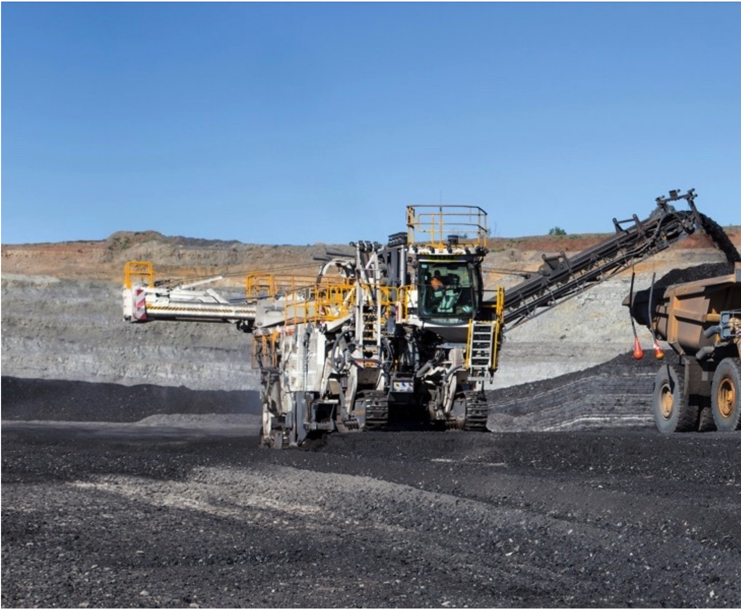
Fig. 1: Wirtgen surface miners – here the 4200 SM – cut and crush the rock with a special cutting drum and load it onto dumpers in a single pass via conveyor system. (Pictures ©Wirtgen GmbH)
