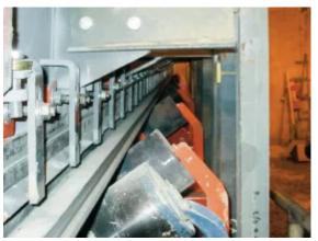
The external skirting system seals the chute to the belt.
