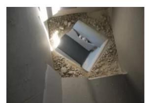
A rock box acts like a shelf, catching and distributing falling material onto the impact cradle.
