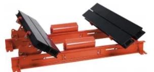
Slider cradles support the belt to prevent spillage from belt sag and eliminate material entrapment points.
