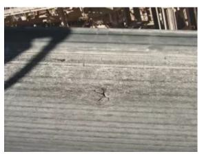
A receiving belt can experience severe damage from material transfers if it's not supported properly. (Pictures: ©Martin Engineering)
