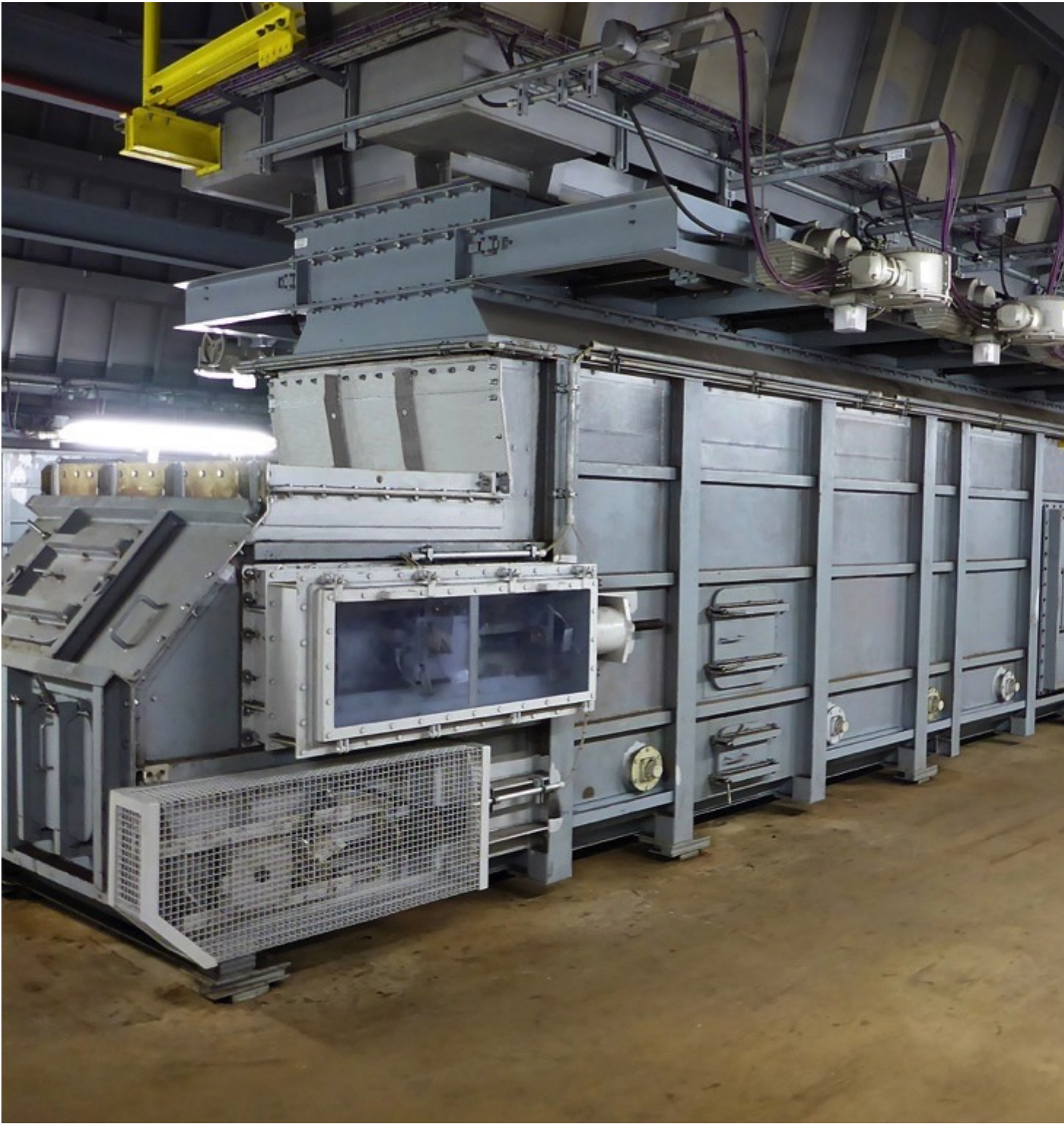
Aumund arched plate conveyors replace the coal feeders at RWE's Neurath power plant. (Picture: © AUMUND Fördertechnik GmbH)
