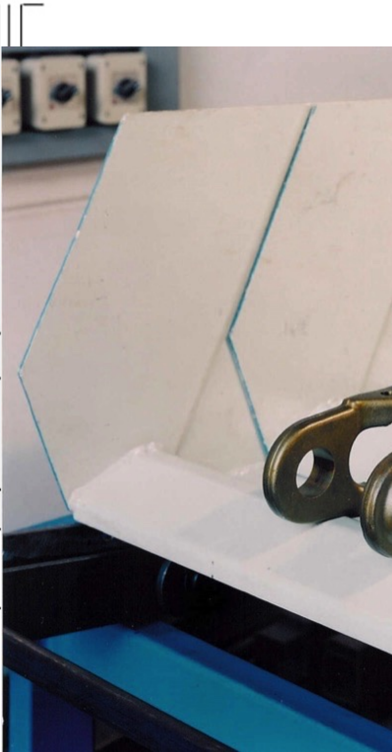
Fig. 4: Elements of an apron conveyor: conveyor cells and chain
