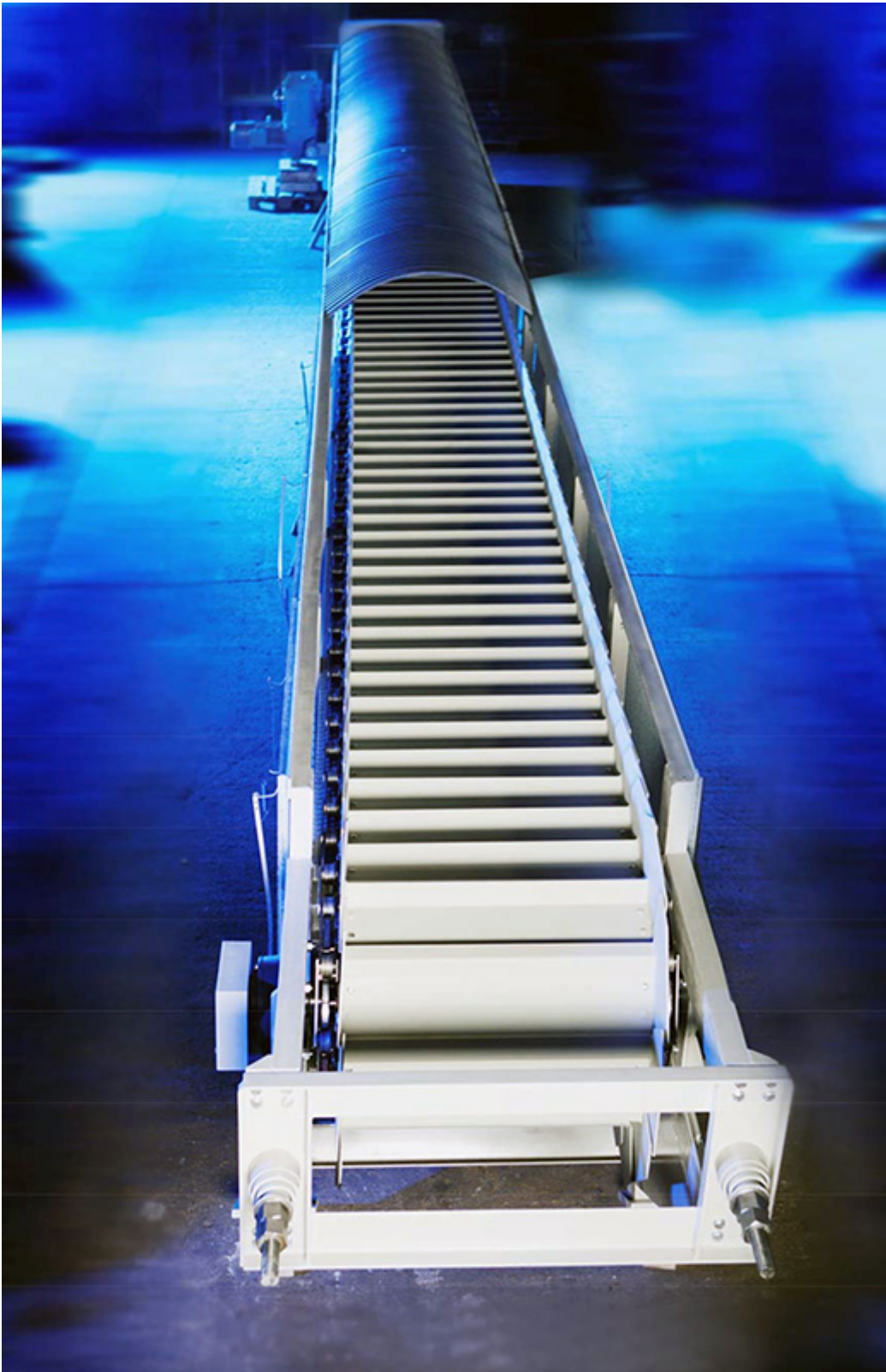
The newly developed Apron conveyor (Picture: Feld-Kleinerüschkamp GmbH)
