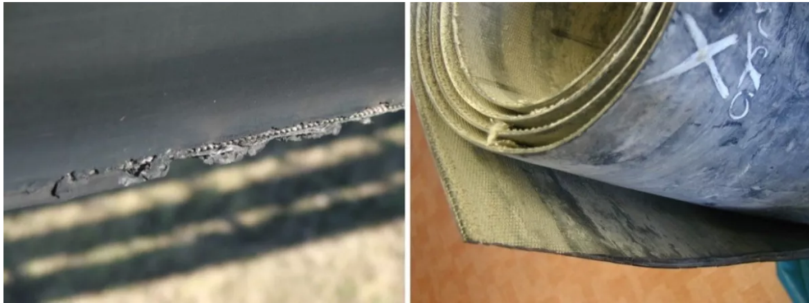
Fig. 1. Example of damage on edge of the pipe conveyor belt. (Pictures: © Technical University of Košice)
