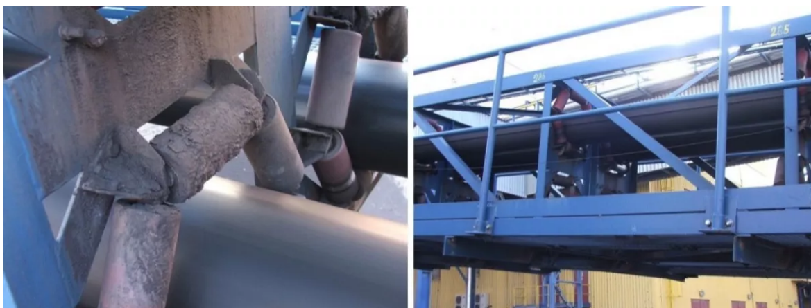
Fig. 2. Example of situation when the conveyor belt does not have a contact with all idler rolls in the hexagonal idler housing.
