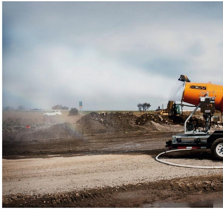
The DB-60 Fusion is powered by an efficient generator for job sites with no utility service.
