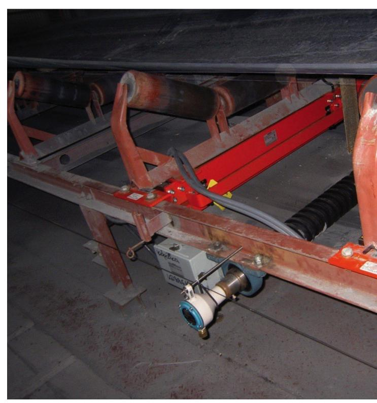
Technicians at the minerals processing plant installed the Milltronics MMI belt scale and Sitrans WS300 speed sensor easily and quickly. (Pictures: © Siemens IS IA)
