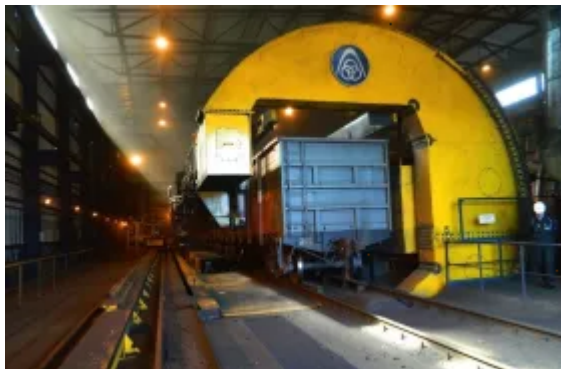
Fig. 1: Tandem tippler working at the Ust Luga coal export terminal, Russia. (Picture ©: ThyssenKrupp India Ltd.)
