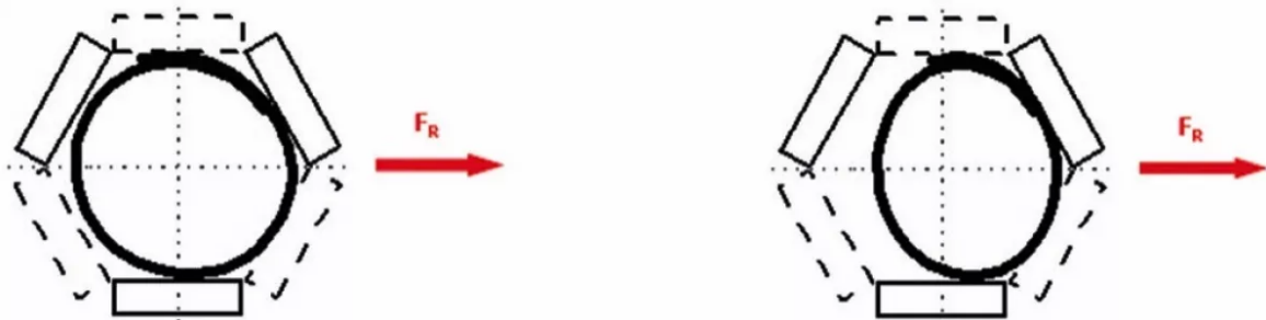
Fig. 8: Sufficient (left) and non-sufficient (right) transverse stiffness.
