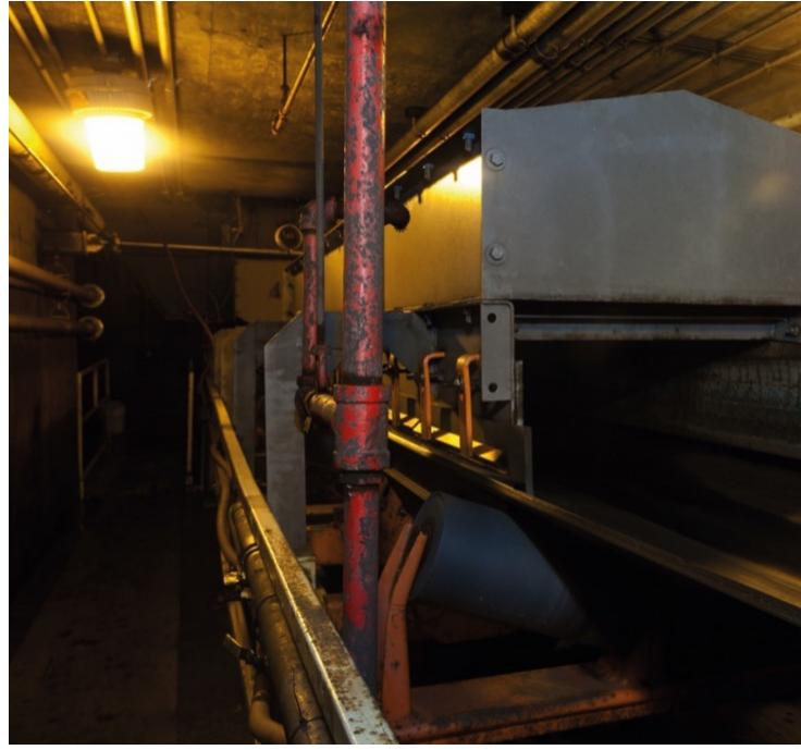
Installed at the bottom of the loading zone skirtboard, Martin Double Apron Seal Skirting employs two wear surfaces on each sealing strip for 2x the service life. (Pictures: © Martin Engineering)
