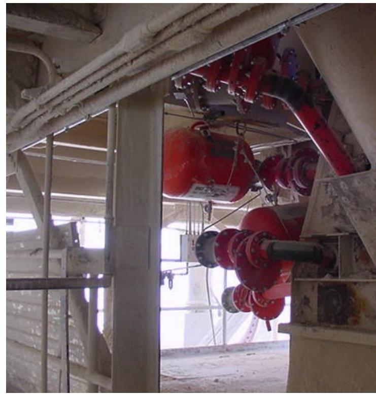
The air cannons in the main production line network are equipped with a negative pressure-firing valve design that delivers reliable operation and long service life in challenging applications.
