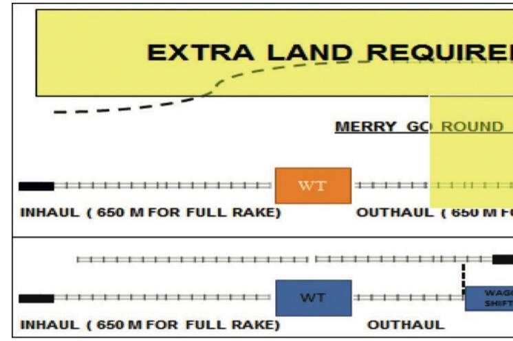
Land requirement for the unloading of coal trains in power stations utilising a wagon tipler together with a merry go round system (above) or a wagon shifter plus pusher system (below).
