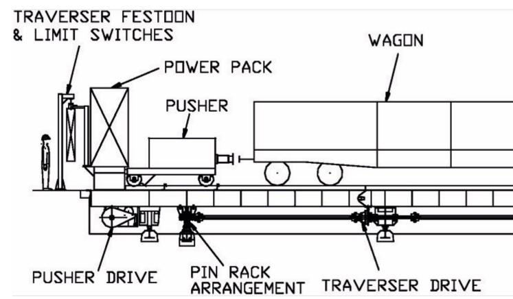
Sketch of the traverser, which runs on three rails.
