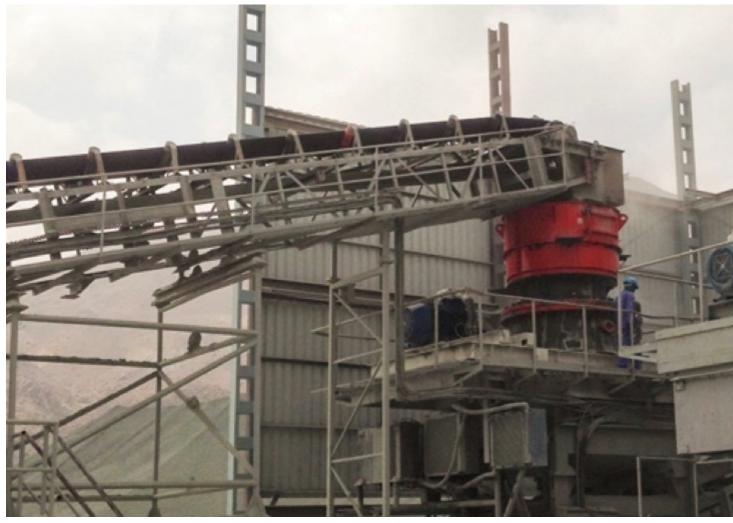
The CH660 cone crusher from Sandvik constrction is at the center of the Raj Rocks LLC aggregate processing plant.
