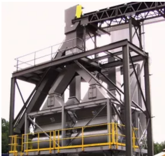
Fig. 10: Metso's Dual AC22.5GI static air-classifier units at Luck Stone's Goose Creek plant, operating at maximum throughput of up to 100 tph. (Picture: © Metso Minerals)
