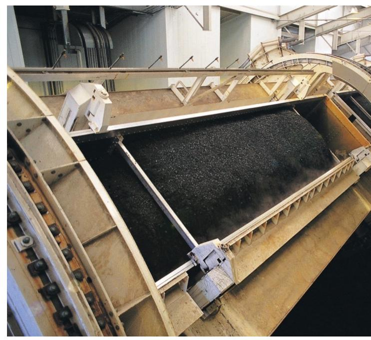
The new dumper system to be delivered to CSX allow for the rotary dumping of loaded railroad cars as well as the unloading of bottom dump cars. (Picture: ©Metso)
