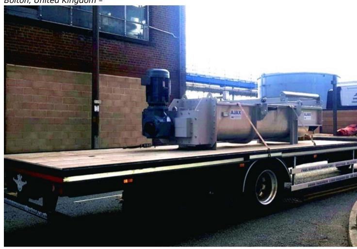
The stainless-steel ash conditioner is based on Ajax's twin screw mixer, ensuring effective mixing and conditioning of the ash, and features spray bars to add acidic liquor.
