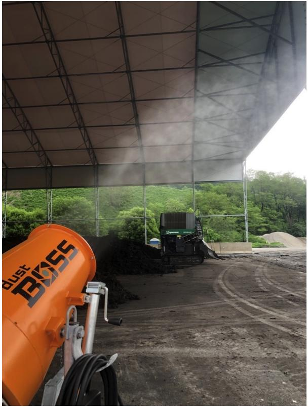
The DB-30 InjektorTM serves dual purposes: suppressing dust and dispersing additives for odor control or disinfection.
