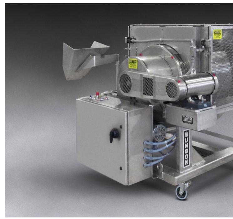
Munson's Rotary Batch Mini Mixer, model MX-5-S316L, blends up to 142  $\ell$  of dry bulk ingredients, with or without liquid additions, in two to three minutes, fully evacuates the batch and sanitises rapidly with no tools.
