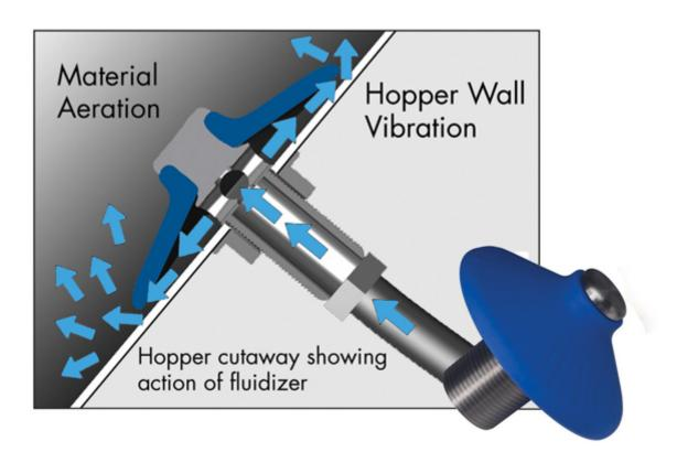
Because cutting holes in silos walls is expensive and time consuming, Solimar's EZ-IN Kits were a natural choice for retrofitting Forpac's eight silos. The system fits existing airpad openings and features a gasket permanently fixed to the mounting plate. Zinc plated carbon or stainless steel models are available in three styles to fit most existing hole patterns.
