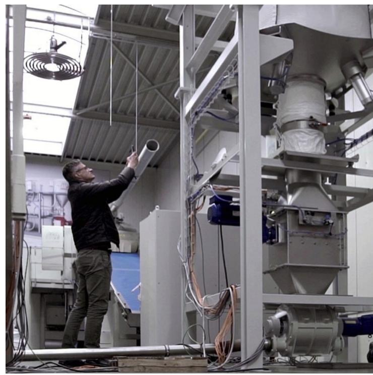
The Dinnissen Big-Bag Conditioner is designed to loosen highly compressed product, resulting in a smooth and fast product flow. (Picture: © Dinnissen Process Technology)
