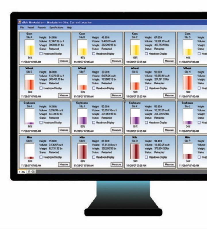
Binventory® works with many types of sensors including non-contact-radar and guided wave radar used for level measurement. The software allows for bulk densities and strapping tables to be entered for solids, while entering specific gravity for liquid tanks ensures spot-on volumes. Complex vessels of different shapes and sizes are easily configured, such as horizontal tanks, split silos, and non-linear tanks.
