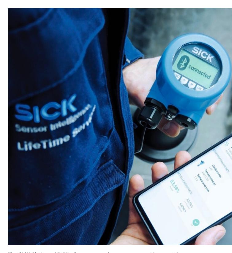
The SICK SicWave 80 GHz free-space radar sensors are a thousand times more sensitive than previous-generation 26 GHz radar technologies, ensuring high availability in even the most challenging environments with minimal maintenance requirements. The narrow field of view also avoids the potential for false signals caused by deposits on walls, or by other obstructions inside the vessel and ensures focused alignment to enable simple and rapid set-up.
