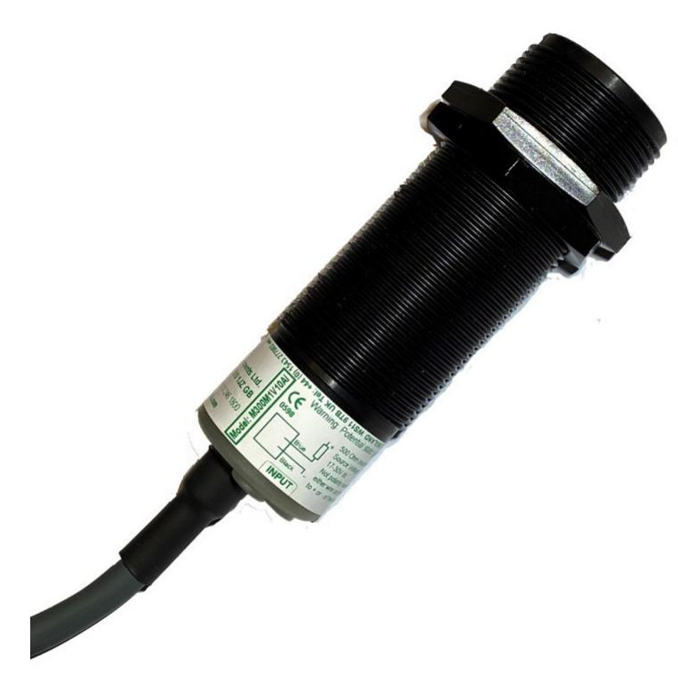
An inductive sensing device located in the nose of the Milli-Speed enclosure will detect a ferrous metal target. This target can be an existing bolt head or device attached to a shaft, such as 4B's Whirligig® sensor mount. During installation, the Milli-Speed is set to the machine's normal running speed by simple magnetic calibration. The 4-20 mA output signal is automatically scaled for zero to full speed with over speed detection.
