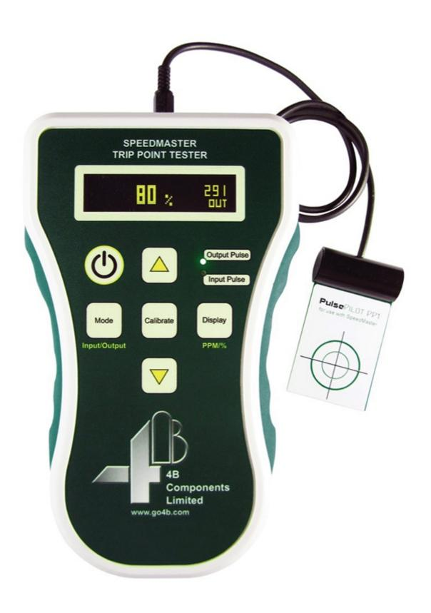
Additionally, 4B's SpeedMaster can be used with the Milli-Speed to test the functionality after the initial installation and during routine maintenance procedures. The SpeedMaster is the only device that accurately tests the calibration of a speed switch, and allows testing of the alarm and shutdown features of the sensor while installed on the machine shaft.
