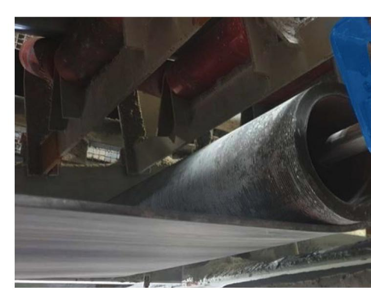
Other advantages include easy installation, low maintenance requirements, and protection of belt edges and structure of the conveyor belt. A strong corrugated EPDM rubber hose protects this system from dust and sand, while the rubber pivot offers soft suspension of the tracker shaft, ensuring extended service life of
