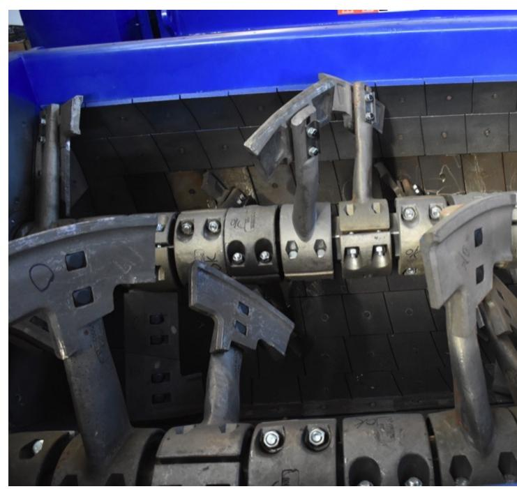
The BHS twin-shaft batch mixer's three-dimensional mixing principle produces a more intensive exchange of material, which leads to shorter mixing times while consuming less energy.
