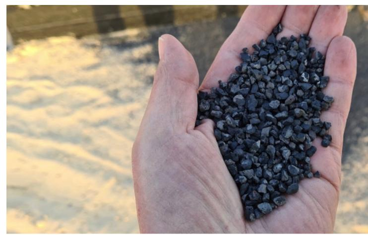
The RSMX produces high-quality slag sand with a particle size of 0 to 4 mm at a throughput of 150 t/h.
