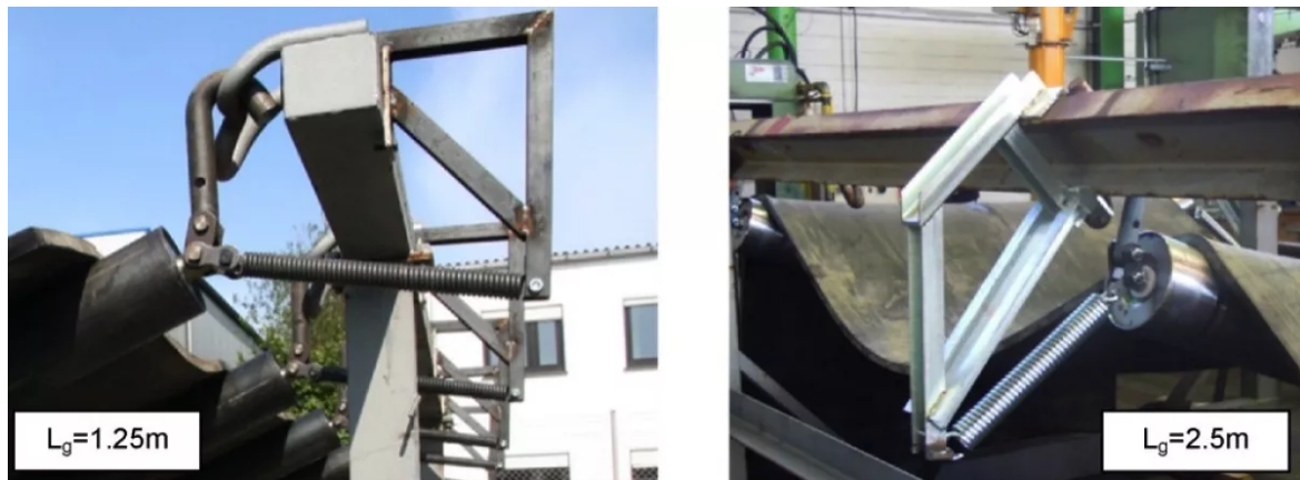
Fig. 6: Different designs of the intelligent garlands suspension depending on garland distance L_g .
