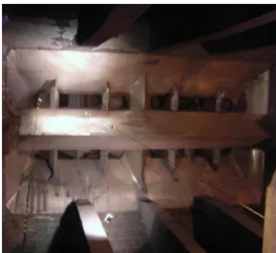
Fig. 4: Two rows of inserts installed in the 1000 tonne section.
