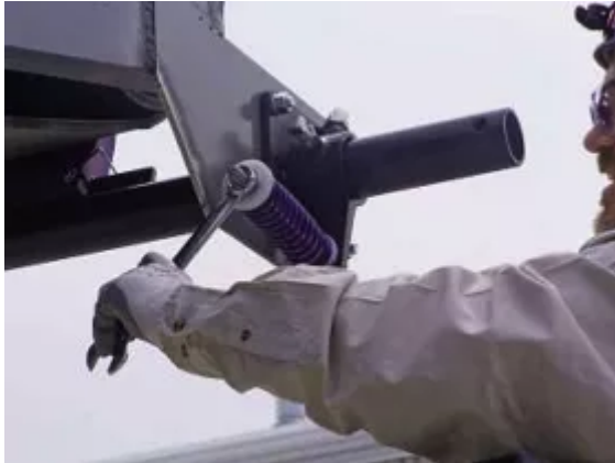
Fig. 4: Fixing a problem with carryback may be as simple as adjusting the tension on cleaners.
