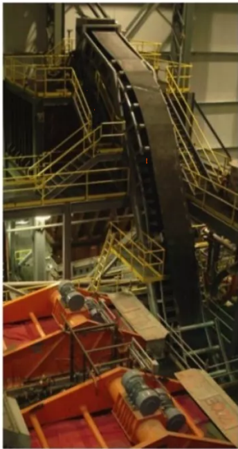
Fig. 10: The third of the three DSI Snake conveyors at the Victoria project – all three conveyors resulted in less building space requirement and save on heating.
