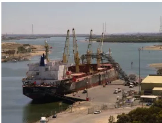
Fig. 11: The DSI Snake ship loader saves space and dock costs.
